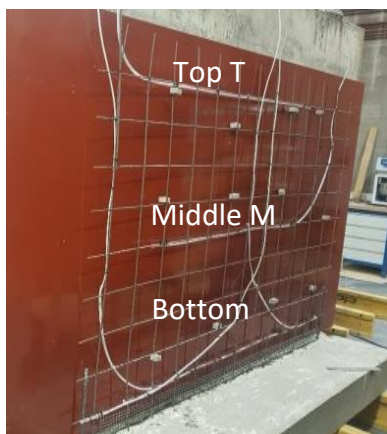
Figure 2: SOFO sensor positions in the concrete wall.
