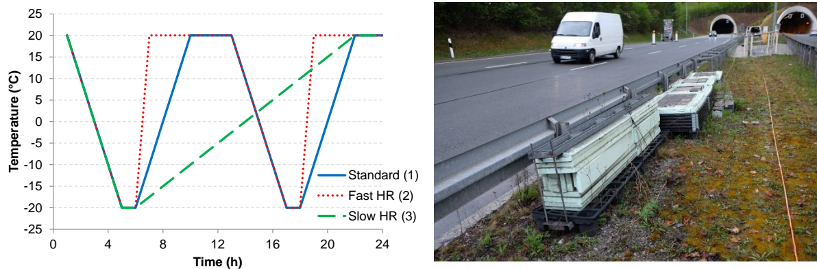
Figure 1: Left: Freeze-thaw cycles of the different series (HR = heating rate); Right: Exposure to field conditions in XF4 (horizontal storage) and XF2 (vertical storage) in Farchant, Germany.
