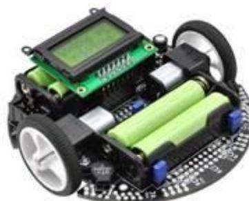
**Figure 6: 3pi line-following vehicle and robot system being developed as test teaching system<sup>3</sup>**
